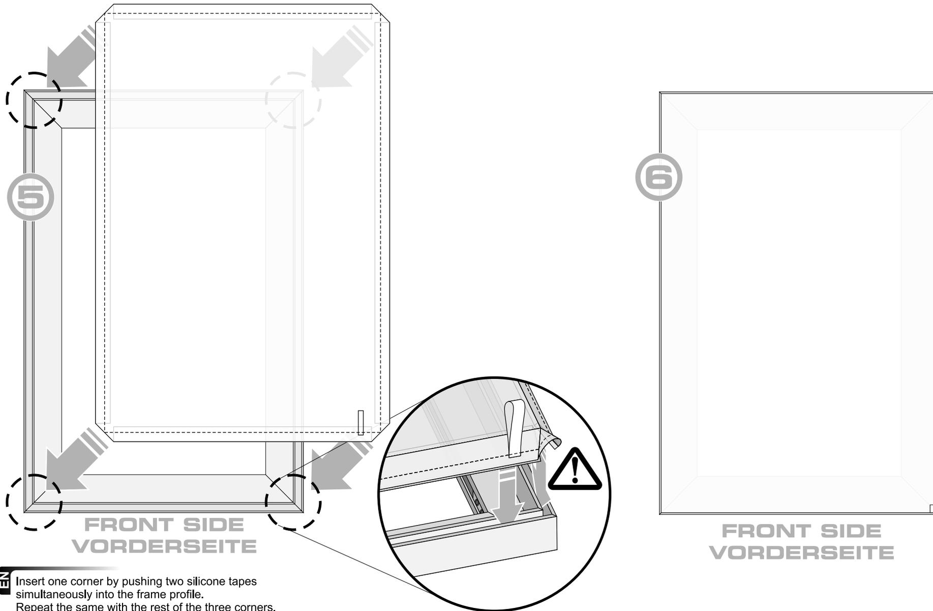
**EN** Insert one corner by pushing two silicone tapes simultaneously into the frame profile. Repeat the same with the rest of the three corners.
